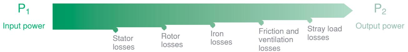
According to IEC 60034-2-1, these losses are obtained with specific methods and efficiency is calculated after loss analysis. Before 2-1 standard issued in September 2007, 60034-2 standard was used for efficiency calculations. The main difference between
